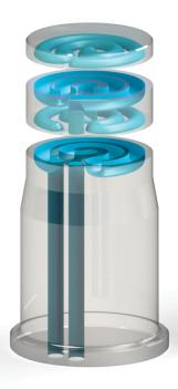
Conformally cooled mold cores and cavities allow molders to make higher quality parts faster.
